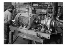
Electric and pneumatic performance testing is performed on repaired industrial and domestic pumps pre-delivery. Dowden's workshop also has a fully equipped tool store with specialised tooling and equipment to perform all works, condition monitoring and laser alignment of pump sets
