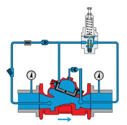
**Valve Open** - At pump start up the energy of the initial surge from the pump start will be arrested by the closed valve, preventing downstream pressure spikes and water surge in the system piping.
