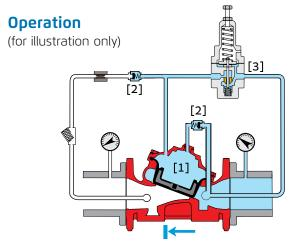
**Valve Closed -** The BERMAD 42T-20 control valve is kept shut tight when the main pump is idle by way of the jockey or maintenance pump pressure held in the valve's control chamber [1] by the check valves [2]. Under the same principle the 42T-20 acts as a system non-return valve, preventing water from flowing back to the main pump after pump shut down.
