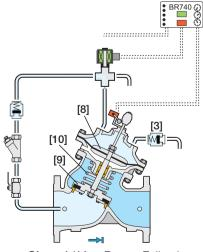
Closed (After Power Failure)
