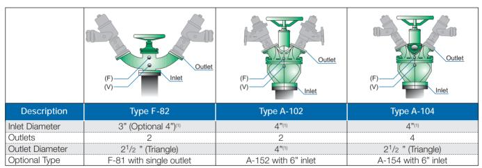
(1) Conforming to major standards (F) Optional port for Automatic Anti-Freezing Cock Valve (V) Optional port for Air Venting Cock Valve
