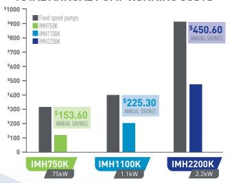
\*Calculation based on typical pump performance data with running time of 5hrs per day with average 40Hz operating speed. 365 days per year at \$0.23 per kWh.
