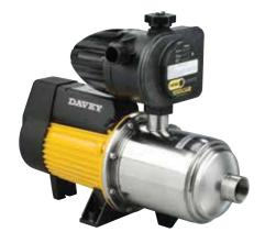
Torrium2 controlled HM Series provides a constant flow water supply system with an all stainless steel pump unit. The Torrium2 is adaptive, eliminating cycling, provides loss of prime protection and over temperature cut out. Pressure tanks can be added if site conditions require additional draw off.
